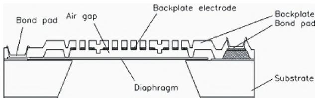
Fig. 1. Cross-section of SiSonic MEMS microphone [1].
