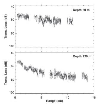
Fig. 2. Measured TL at two receiver depths (60 and 120 m). The results for all eleven frequencies are shown.
