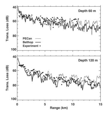
Fig. 4. Comparison of measured and modelled transmission loss at a single frequency (1010 Hz).
