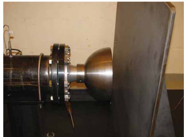
Figure 2. Jet Nozzle with bell mouth.
