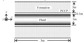
Figure 1. Typical model geometry with dimensions.
