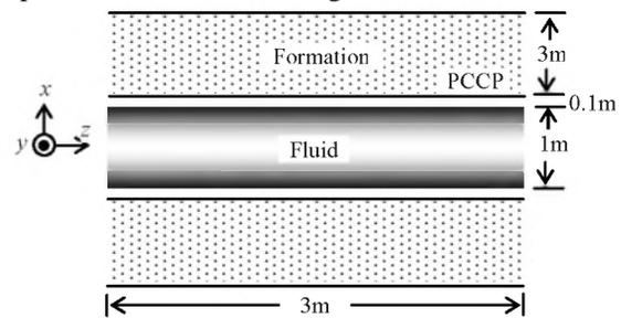
Figure 1. Typical model geometry with dimensions.
