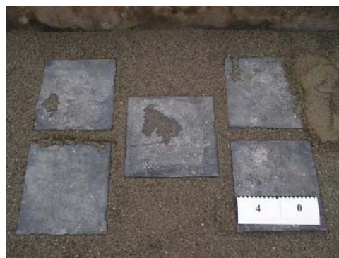
Fig. 4: Structural Isolation Pads, immersed in Compacted Sand
