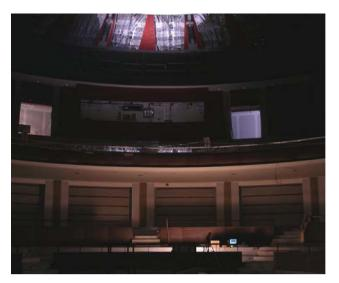
Figure 4. Illustration of light source being used to test the aiming of reflectors. Light behind camera aimed at reflectors at top, reflects to balcony seating, centre (foreshortened).
