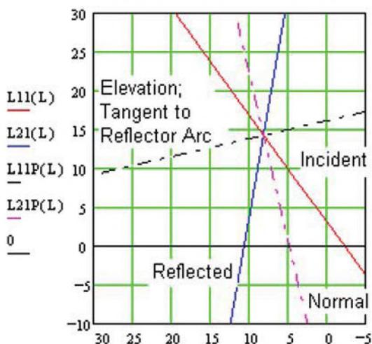
Figure 3. Graphic Output from MathCAD Reflection Routine
