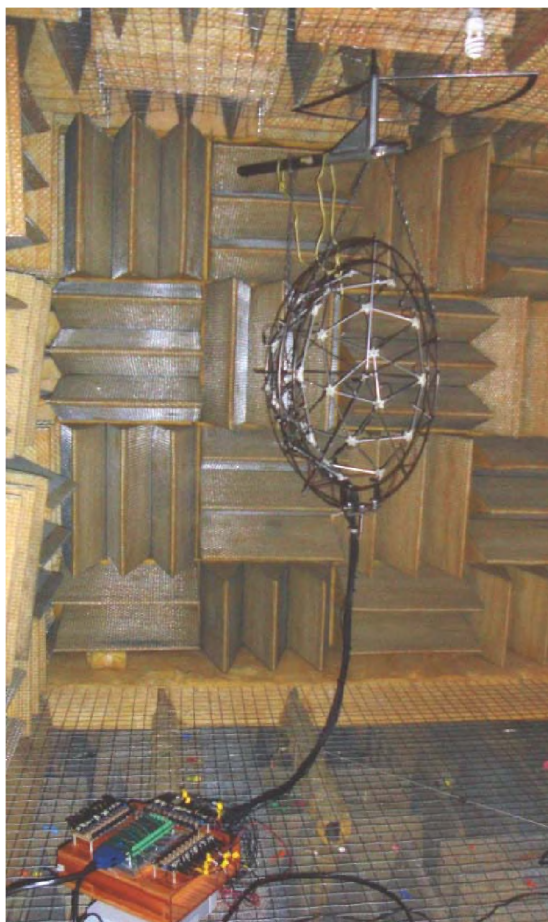
Figure 1. Antenna and DAQ system in anechoic chamber.
