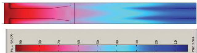
Figure 2. Sound Propagation inside Silencer #2 @ 1050 Hz.
