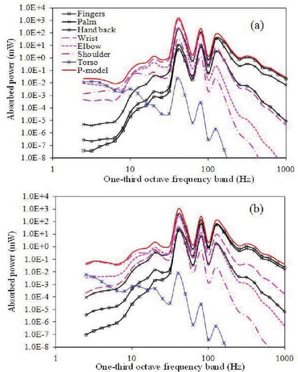
**Figure 2. Distributed and total power absorbed in the human hand-arm due to chipping hammer excitation: (a) bent-arm posture; (b) extended-arm posture.**
