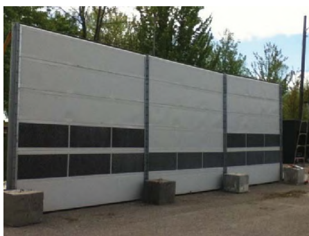
Figure 1. Experimental on-scale sound barrier wall
