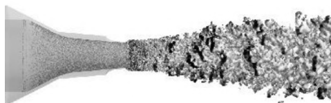
Figure 1. SMC nozzle: 0.9 jet Q-criterion isosurface.
