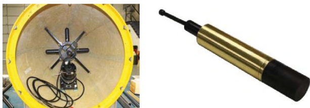
Figure 3. Digital LRAB Array mounted in AUV nose cone (left), Deep water digital hydrophone (right)
