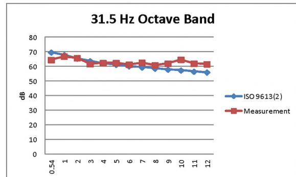
Figure 1 Comparing Model & Measurements at 31.5 Hz
