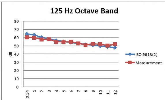
Figure 3 Comparing Model & Measurements at 125 Hz
