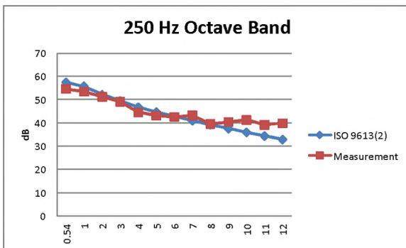
Figure 4 Comparing Model & Measurements at 250 Hz
