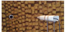
Fig. 2: Electro acoustic tests performed on 3D prints to validate the mechanical design of the body
