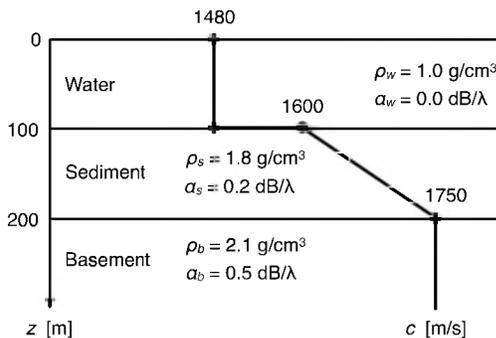
Figure 1. Pekeris type waveguide with a sediment layer.
