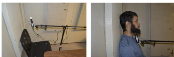
Figure 5: Probe setting with non-participant human model
