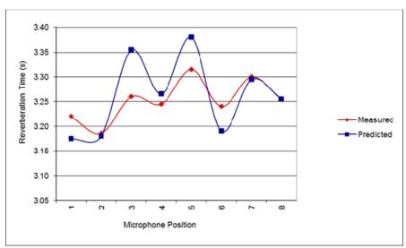
Figure 4. Measured and predicted reverberation times ( $T_{500+1000Hz}$ ) for Loudspeaker position S2
