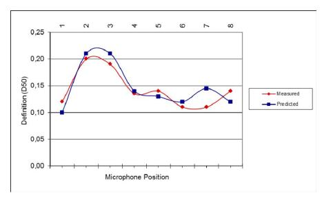
Figure 9. Measured and predicted values of Definition  $(D_{50})_{(500+1000) \text{ Hz}}$  for Loudspeaker position 1.
