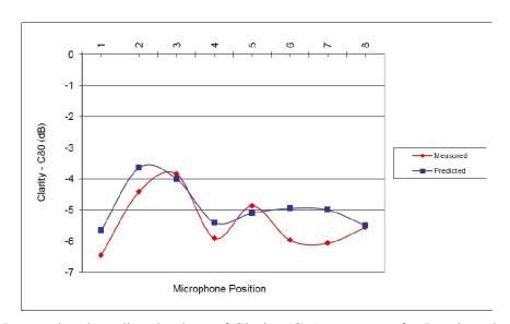
Figure 7. Measured and predicted values of Clarity (C<sub>80</sub>) (500+1000 Hz) for Loudspeaker position 1
