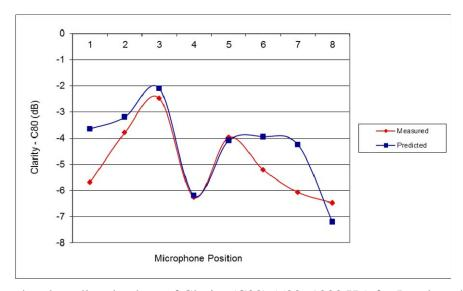
Figure 8. Measured and predicted values of Clarity (C80) (500+1000 Hz) for Loudspeaker position 2
