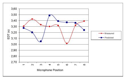
Figure 6. Measured and predicted Early Decay Times (EDT<sub>500+1000 Hz</sub>) for Loudspeacker position S2
