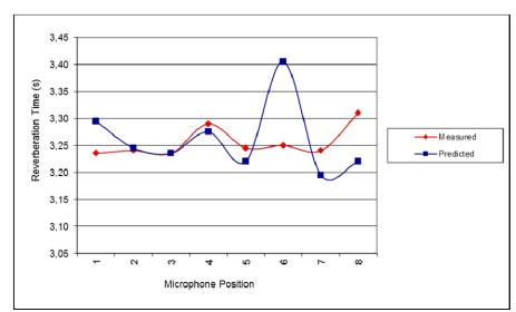
Figure 3. Measured and predicted reverberation time ( $T_{500+1000Hz}$ ) for Loudspeaker position S1
