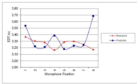
Figure 5. Measured and predicted Early Decay Times (EDT<sub>500+1000Hz</sub>) for Loudspeaker position S1
