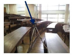
Figure 8: Position of the sound level meter at the students' seats.
