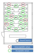
**Figure 16:** Floor plan of room PG 06, showing the location of the measuring points and the values of  $D_{50}$ , in percent [%]. The *green color* shows the points within the range of 39% to 67%, which are considered *Fair*, according to Marshall [11].
