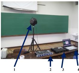
**Figure 7:** Equipment for measuring RT and D50: 1) Omnidirectional sound source; 2) Fireface 800 audio interface; 3) Power amplifier; 4) Notebook with Dirac software.
