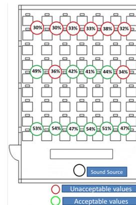
**Figure 15:** Floor plan of room PG 04, showing the location of the measuring points and the values of  $D_{50}$  in percent [%]. The green color shows the points within the range of 39% to 67%, which are considered *Fair*, according to Marshall [11].
