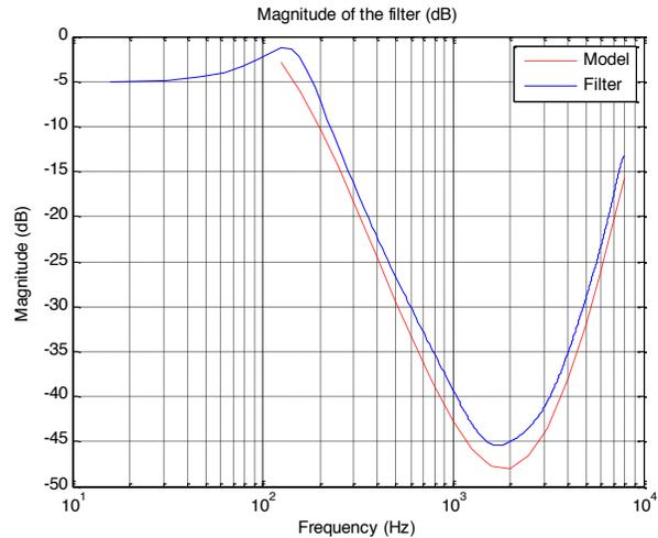
**Figure 12: Frequency response of the filter (in blue)**
