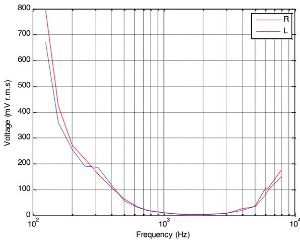
**Figure 10: Bone transducers input voltage for a "flat" uniform bone stimulation – Left transducer in blue and right transducer in red**
