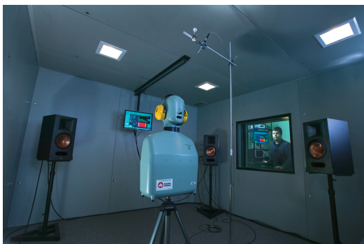
Figure 3: Double wall audiometric test booth
