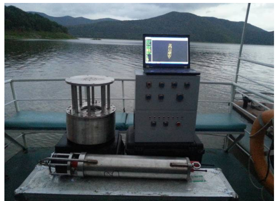
Figure 1: Components of the LBL system tested in the field trial, including transducer, transponder, computer, signal processing box and power box (counter-clockwise from top left)
