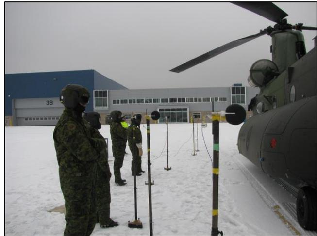
Figure 2: Exterior Noise Measurement
