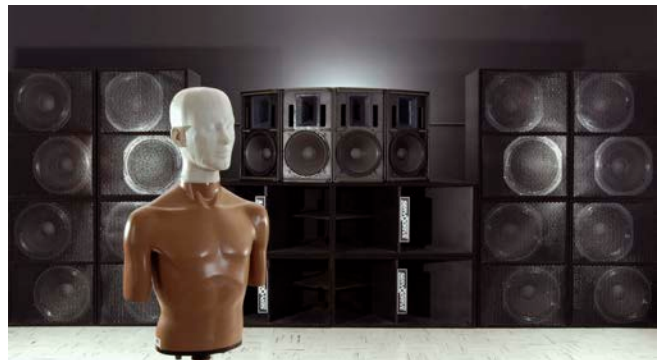
Figure 1: Speaker system and acoustic manikin in the Noise Simulation Facility. Photo credit: Jim Clark.
