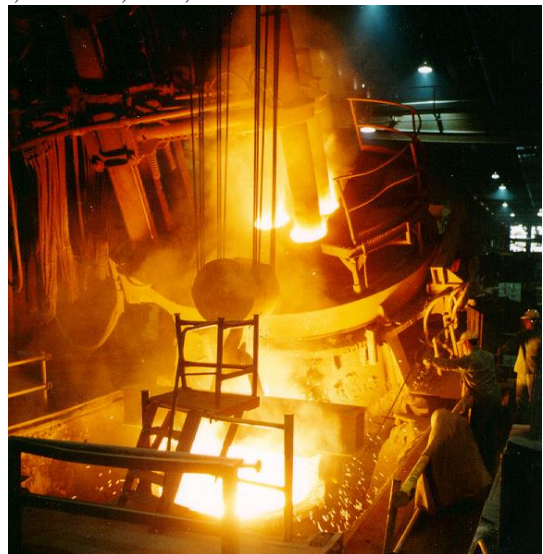
Figure 2. Electric Arc Furnace - Typically >110 dBA @ 10m
