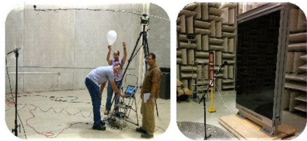
Figure 3: On-site measurement of a reverberation time and noise characterization of a digital display unit in the semi-anechoic chamber.
