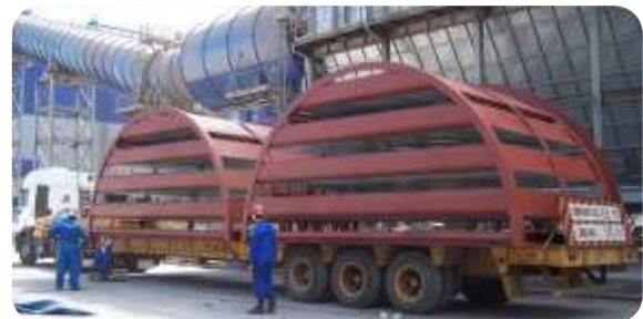
Figure 2: Stack Silencer for South American Power Plant
