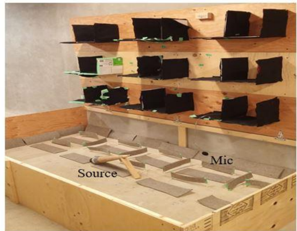
Figure 1. Photograph of the model (open roof) with workstations showing source, receiver and sound absorbers.
