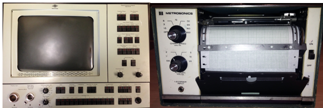
Figure 2: Brüel and Kjør 1233 Real Time Analog Frequency Analyzer (left) and Metrosonics Chart Recorder (right)
