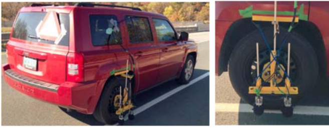
Figure 2: AASHTO-complaint OSBI Test Rig Used in Measurements
