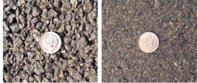
Figure 1: Open graded pavement (OGFC) versus Typical Control pavement (Superpave HMA)
