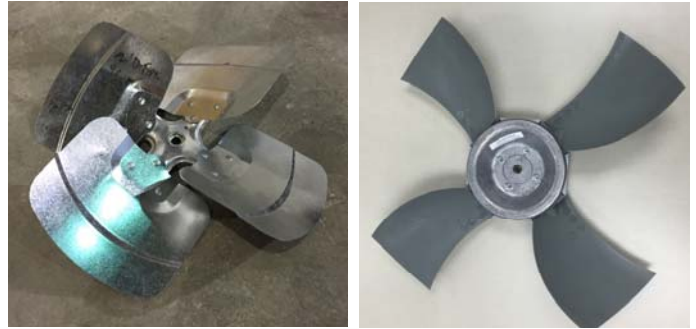
Figure 4: Original and Final Replacement Fan for PTAC Units
