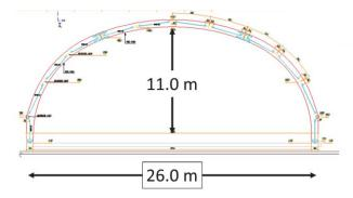
Figure 3: Section of the air dome
