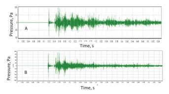
**Figure 19:** (A) Impulse response of the central point obtained with the Odeon software, without acoustic correction. (B) Impulse response when sound absorbing material for acoustic correction is applied under the dome.
