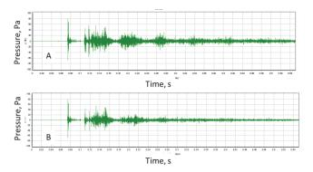
**Figure 18:** (A) Impulse response of the central point obtained with the Odeon software, without acoustic correction. (B) Impulse response when sound absorbing material for acoustic correction is applied under the dome.
