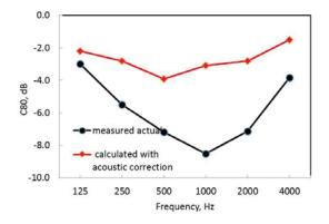
**Figure 17:** Comparison between  $C_{80}$  measured versus calculated with acoustic correction
