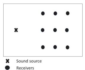
Figure 4: Plant with the indication of the sound source (X) and receivers (microphones) (o).
