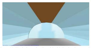
Figure 14: 3D air dome virtual model with the absorbent panels under the vault
