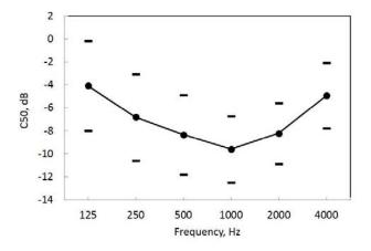
**Figure 7:** Measured average values of  $C_{50} \pm 1$  standard deviation.
