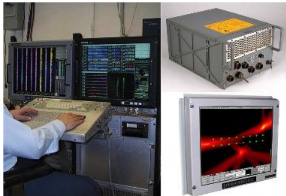
Figure 2: Left: IMPACT – airborne concept demonstrator; right: MVASP processor (top) and display (bottom).
