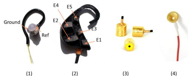
Figure 2: Electrodes used for this study: EARtrodes' custom-fitted earplug (1) and behind-the ear piece (2), gold foil electrodes (3) and gold-plated cup electrodes (4).
