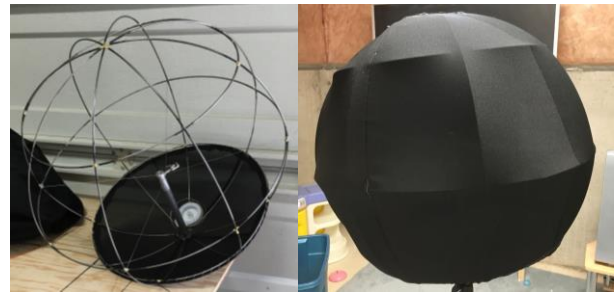
Figure 1: Secondary windscreen shown with and without speaker grill cloth cover.
