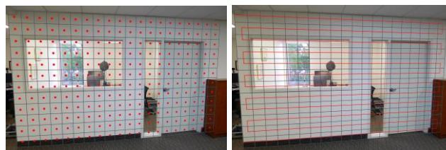
Figure 1: Grid with discrete points (left) and scanning path (right)
