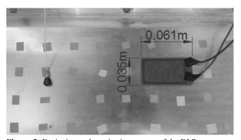
**Figure 5:** Excitation and monitoring system of the DLR test setup, using a piezoelectric patch and an accelerometer.
