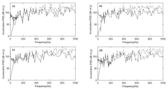
**Figure 9:** Comparison, using Berry's model, of predicted (solid line) vs. experimental (dashed line) of acceleration PSD results for a panel with arbitrary boundary conditions: (a) measured at (M): x = 26.2 cm, y = 8.6 cm with a piezoelectric actuator excitation applied at (F): x = 12.3 cm, y = 7.4 cm (b) M: x = 31.4 cm, y = 26.0 cm and F: x = 12.3 cm, y = 7.4 cm (c) M: x = 31.4 cm, y = 26.0 cm and F: x = 15.5 cm, y = 26.0 cm (d) M: x = 25.5 cm, y = 13.4 cm and F: x = 15.5 cm, y = 26.0 cm
