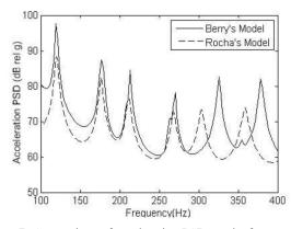
**Figure 7:** Comparison of acceleration PSD results for a panel with simply supported boundary conditions at a point x=a/4 and y = b/4, with a TBL excitation applied. Each target frequency is calculated with the same constant number of panel modes (m, n) = (9,7).
