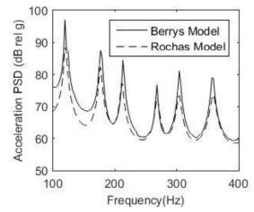
Figure 6: Comparison of acceleration PSD results for a panel with simply supported boundary conditions at a point x=a/4 and y = b/4 with a TBL excitation applied.
