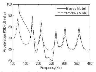
**Figure 8:** Comparison of acceleration PSD results for a panel with simply supported boundary conditions at a point x=a/4 and y = b/4, with a TBL excitation applied. Each target frequency is calculated with the same constant number of panel modes (m, n) = (14, 11).
