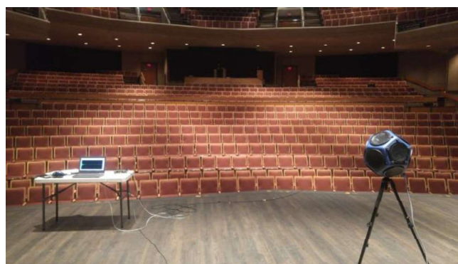
Figure 2: Room acoustics measurements in a concert hall with an omni-directional source
