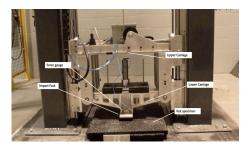
Figure 2: Heavy Weight Drop Tower at rest
