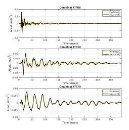
Figure 4: Predicted vs Measured Vibration in Time Domain
