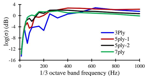
**Figure 3:** Simulated RE of Canadian CLT plates.
