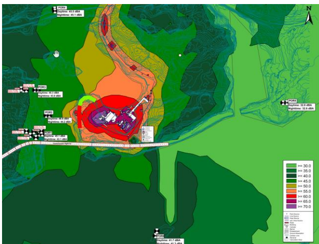
Figure 3: Model indicating non-impulsive noise levels after implementation of log barrier (red) and earth berm (green).
