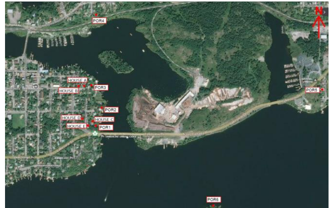
Figure 1: Log processing facility in the centre, with receptor locations shown in red indicating residential communities impacted by noise
