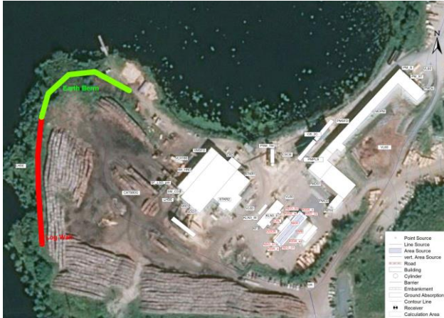
Figure 2: Proposed noise barrier consisting of a log wall (red) and an earth berm (green).
