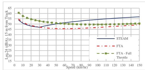
**Figure 4:** Total  $L_{eq,24hr}$  as a function of Speed, STEAM vs. FTA
