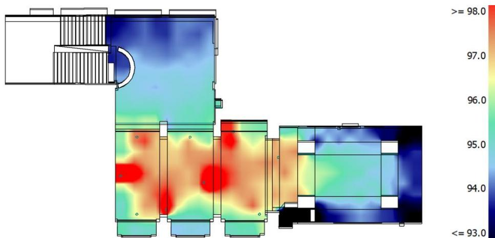
**Figure 10:** Simulated values of A-weighted sound pressure level (SPL(A) in dB(A)) in the occupied condition with nine loudspeakers active (see fig. 5).
