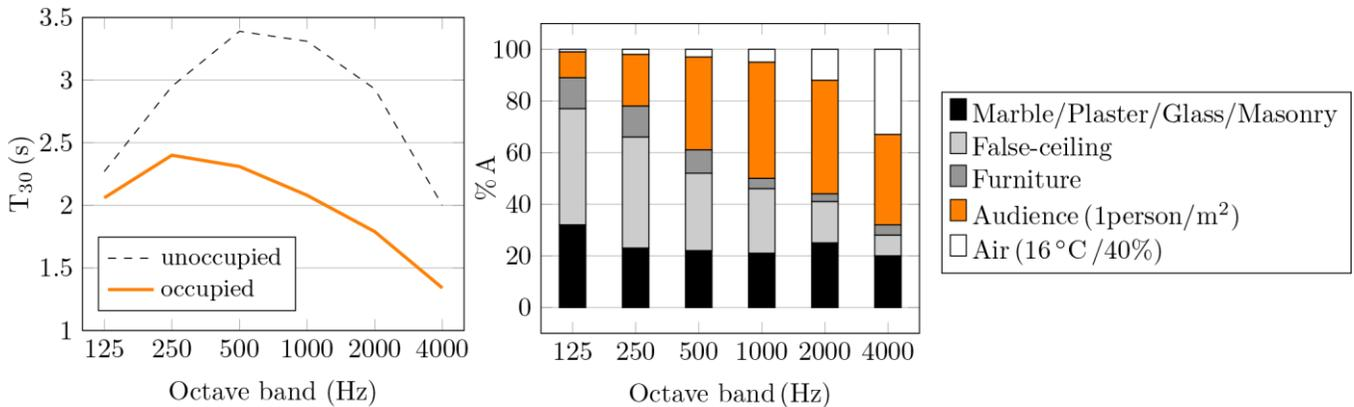
**Figure 7:** On the left, mean values of simulated reverberation time ( $T_{30}$ ) in the unoccupied and occupied conditions. On the right, percentages of equivalent absorption area (% A) of the materials involved in the simulations
