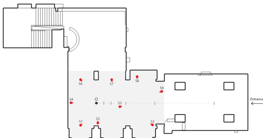
**Figure 5:** Plan of the atrium of the historical building under study: positions of the sound sources (S1 - S9) set by Florian Hecker during his sound performance. IRs were measured in the calibration process, placing omni-directional sound source (O) and receivers along the dashed line. Grey zone corresponds to the audience area during the performance (see fig. 2).
