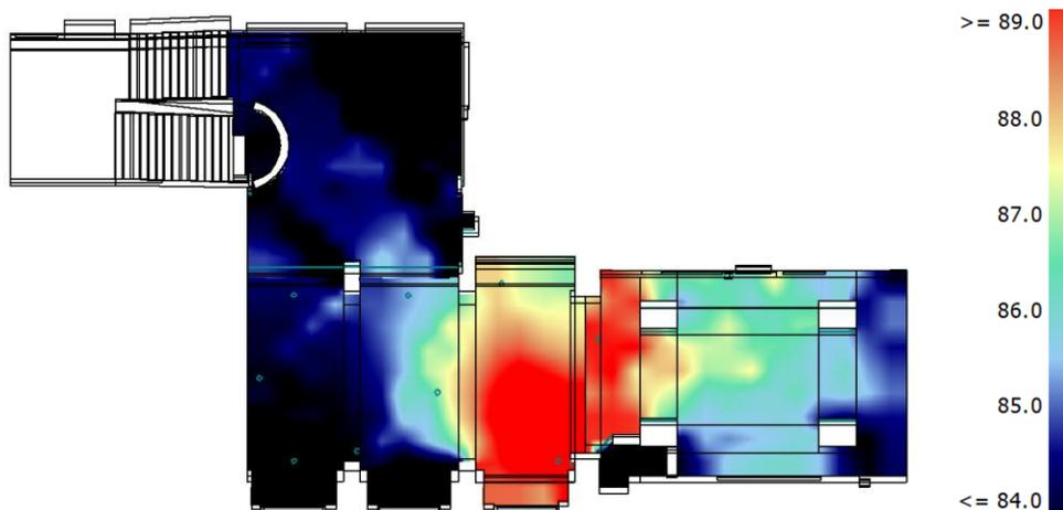
**Figure 9:** Simulated values of A-weighted sound pressure level (SPL(A) in dB(A)) in the occupied condition with the loudspeaker S3 active (see fig. 5).
