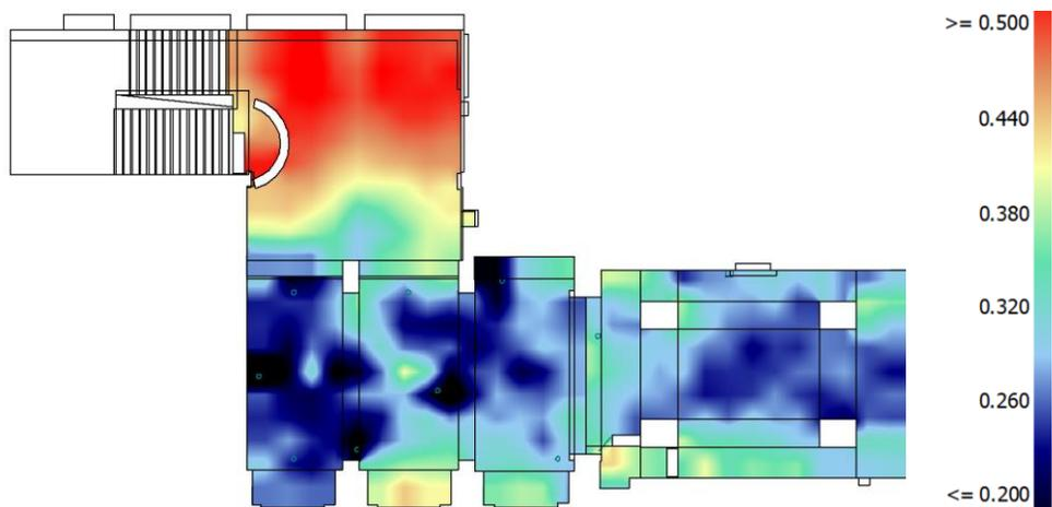
**Figure 11:** Simulated values of lateral fraction ( $LF_{80}$ ) at 500 Hz in the occupied condition.
