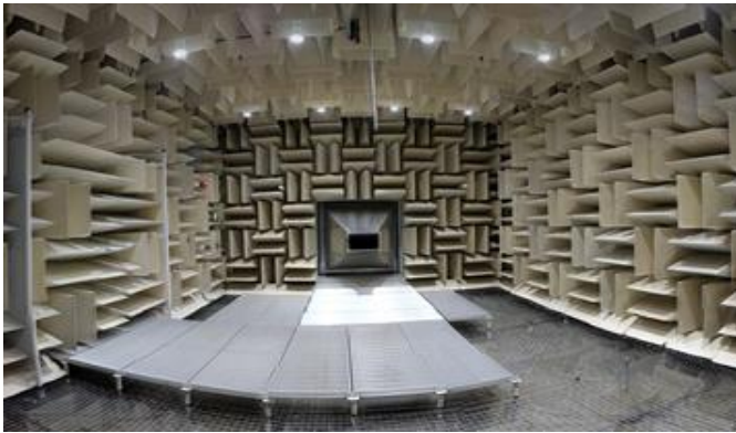
Anechoic room and wind-tunnel opening at GAUS
