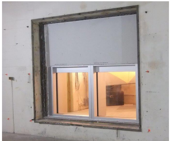
Figure 2 : Window Specimen prepared for STC-testing, showing Filler Wall above Specimen
