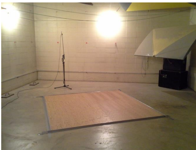
Figure 1: Specimen prepared for ASTM C423 testing.
