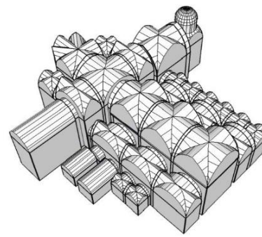
Figure 4: 3D model of the church used to test possible interventions for its acoustic correction.
