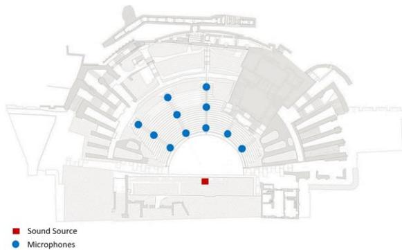
**Figure 6:** Measurement setup: red point indicates the sound source position and the blue points indicate the receiver positions.
