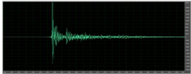
**Figure 7:** Measured IR in the Roman theatre of Verona having the sound source placed in the *proscenium* and the receiver (omnidirectional microphone) placed in the central sector of the *summa cavea*.
