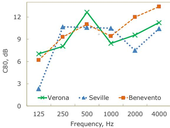
Figure 10: Measured results of Clarity Index ( $C_{80}$ ).
