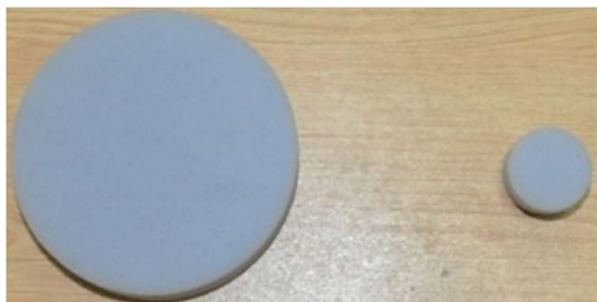
Figure 5: Testing samples of melamine foam (100 mm & 30 mm diameters)
